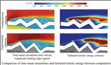
and experiment at  $\text{Re}_c = 3.4 \times 10^4$  and angle of attack= 5°
